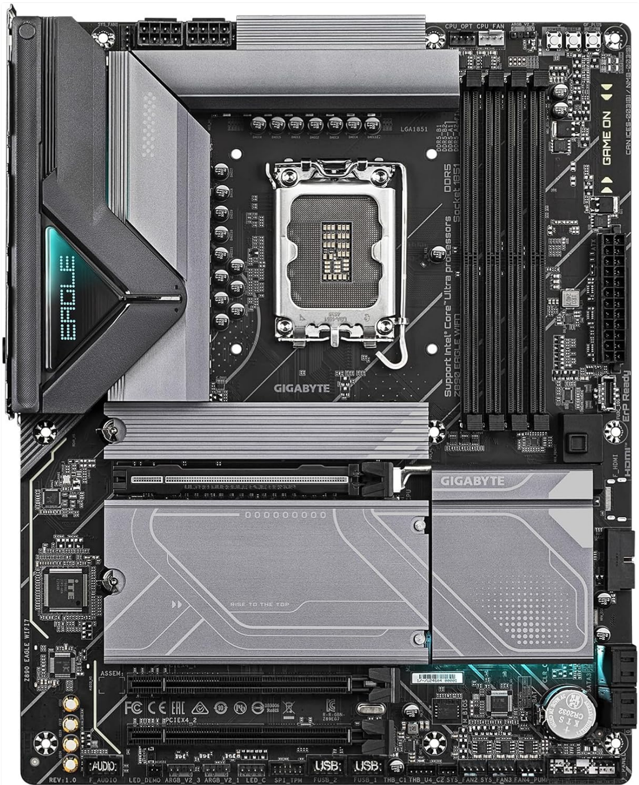
Figure 2: Close-up of the LGA 1851 CPU socket on the motherboard.
