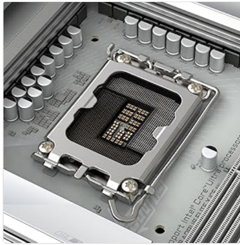
Figure 2: Close-up view of the LGA 1851 CPU socket.
