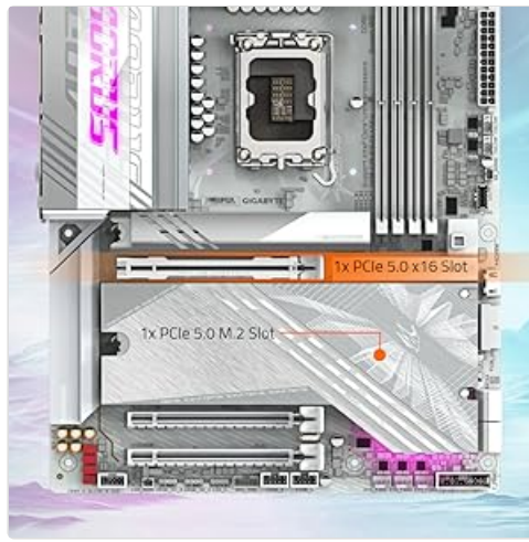
Figure 4: PCIe 5.0 and M.2 slots with EZ-Latch feature.
