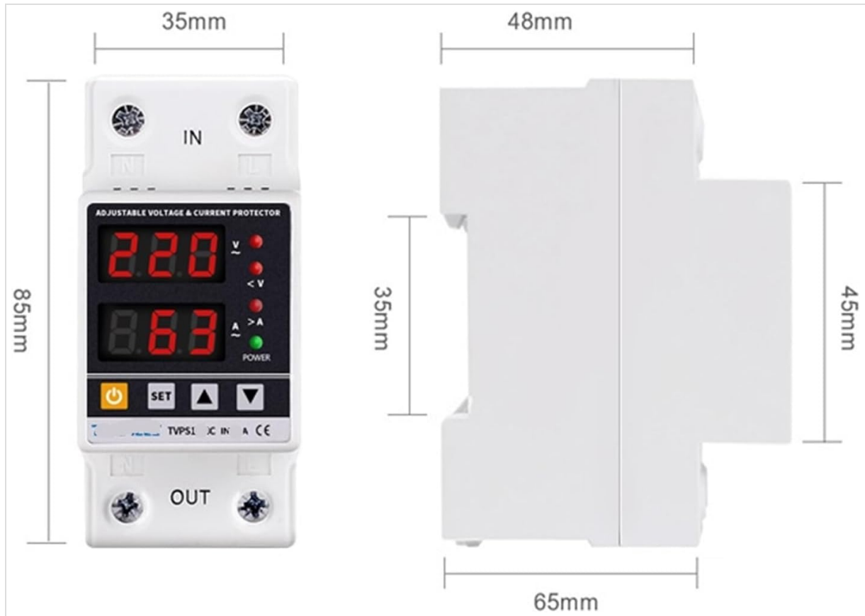
Figure 2: Dimensions of the AVXANKTG TVPS1-63 protector. The front view shows a width of 35mm and height of 85mm. The side view shows a depth of 65mm and a height of 45mm for the main body, with the DIN rail clip adding to the total height.
