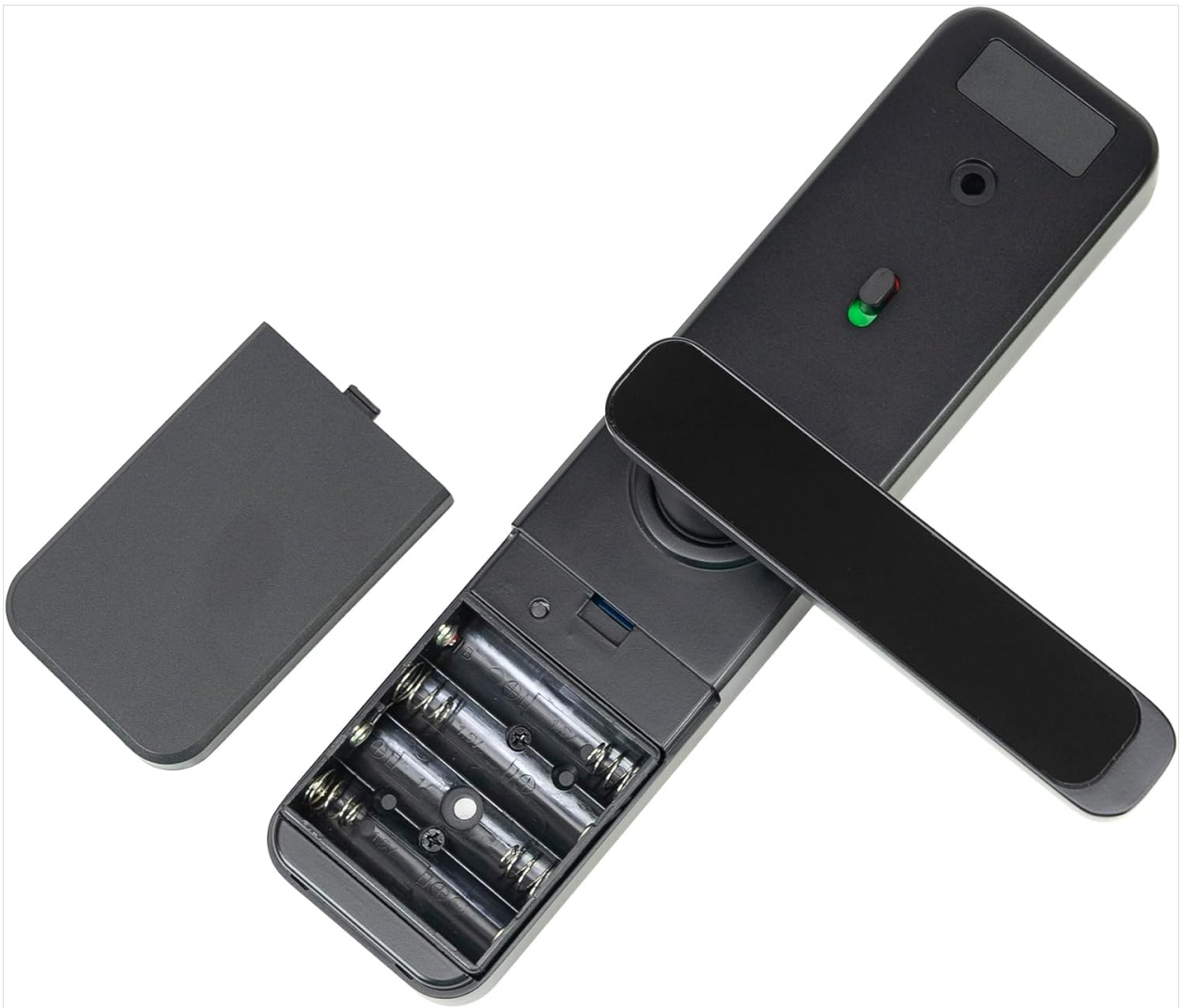
Image 4.1: The battery compartment located on the interior side of the lock, showing slots for four AA alkaline batteries.
