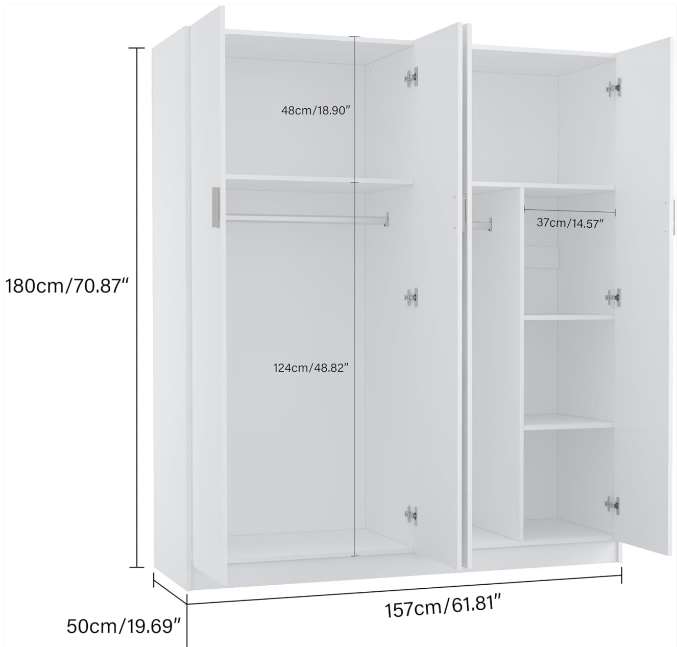
Figure 7.2: Interior and overall dimensions of the Panana U104 Wardrobe.
