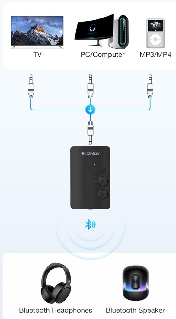
Image: A diagram illustrating how to connect the adapter in both Transmitter (TX) and Receiver (RX) modes to various audio devices.
