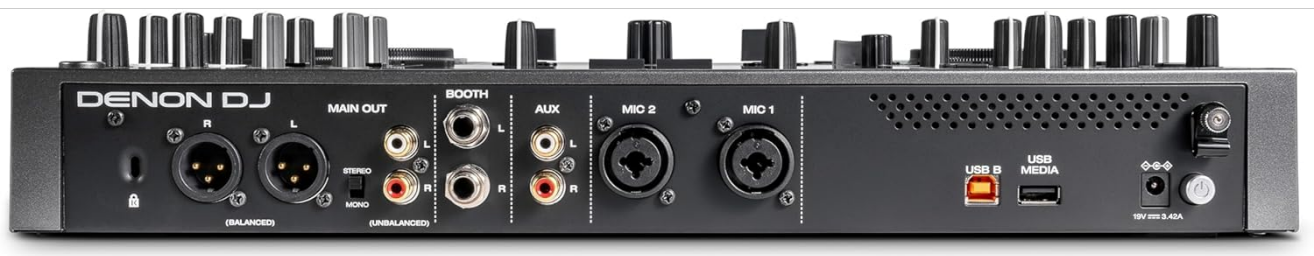
Figure 9: Actual view of the rear panel connections, showing main outputs, booth outputs, AUX inputs, mic inputs, USB ports, and power input.
