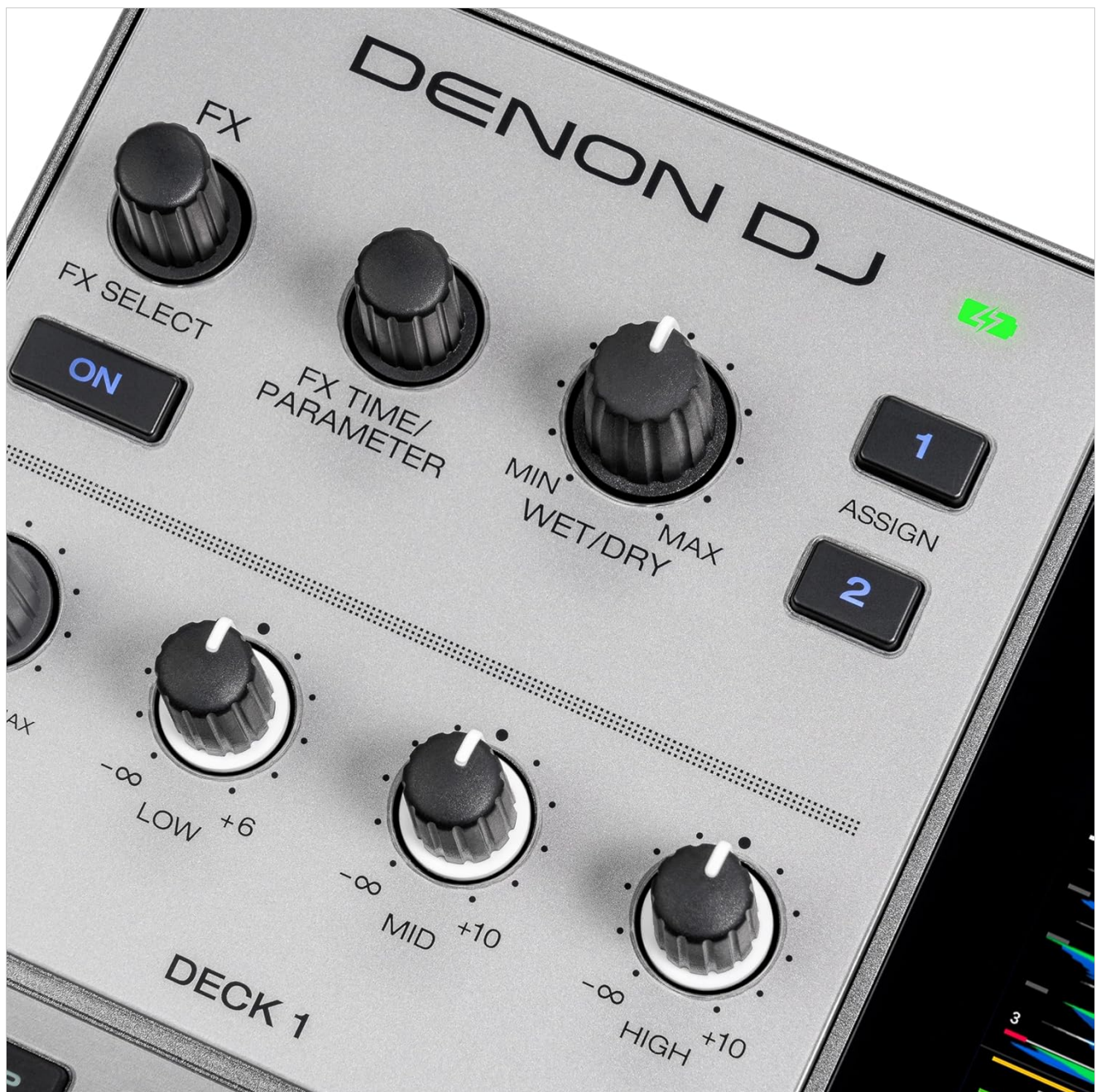
Figure 14: Close-up of the FX section, showing FX select buttons, parameter knobs, and wet/dry control.
