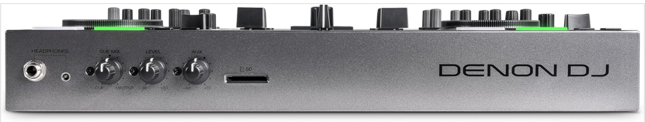
Figure 10: Actual view of the front panel connections, including headphone jacks, cue mix, level, AUX controls, and SD card slot.
