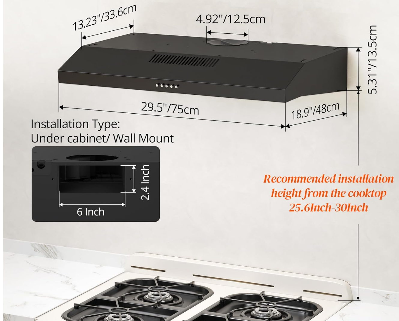
Figure 8: Detailed dimensions of the range hood and recommended installation height above a cooktop.
