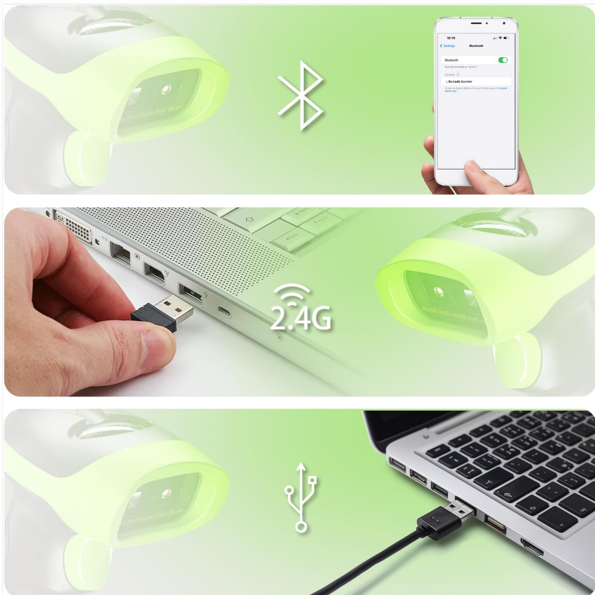
Image 2: Illustration of the three connection methods: Bluetooth pairing with a smartphone, inserting a 2.4G USB dongle into a laptop, and connecting via USB cable to a laptop.
