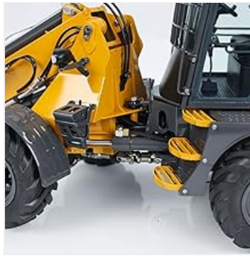
Image: Detailed view of the hydraulic steering components, showing the articulation for precise control.
