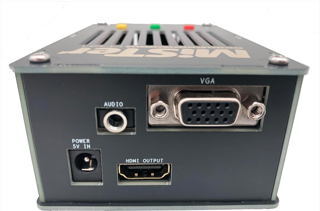
Figure 2: Rear view of the QMTECH Mister FPGA unit, displaying the POWER 5V IN port, 3.5mm Audio jack, VGA output port, and HDMI output port for display connectivity.
