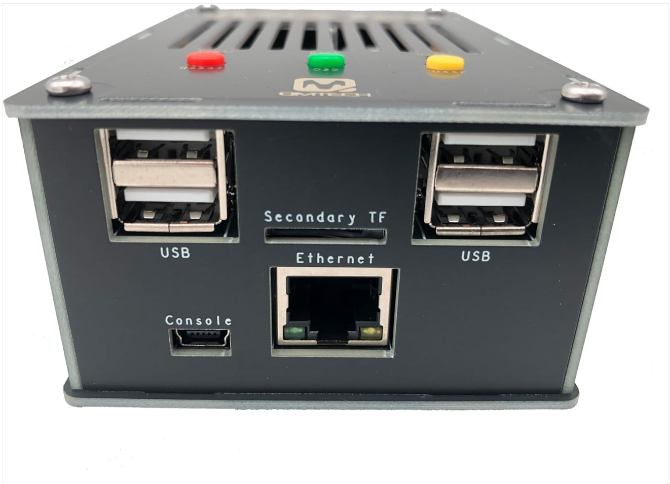
Figure 3: Side view of the QMTECH Mister FPGA unit, featuring two USB ports, a Secondary TF card slot, an Ethernet port, and a Console port for various connections.
