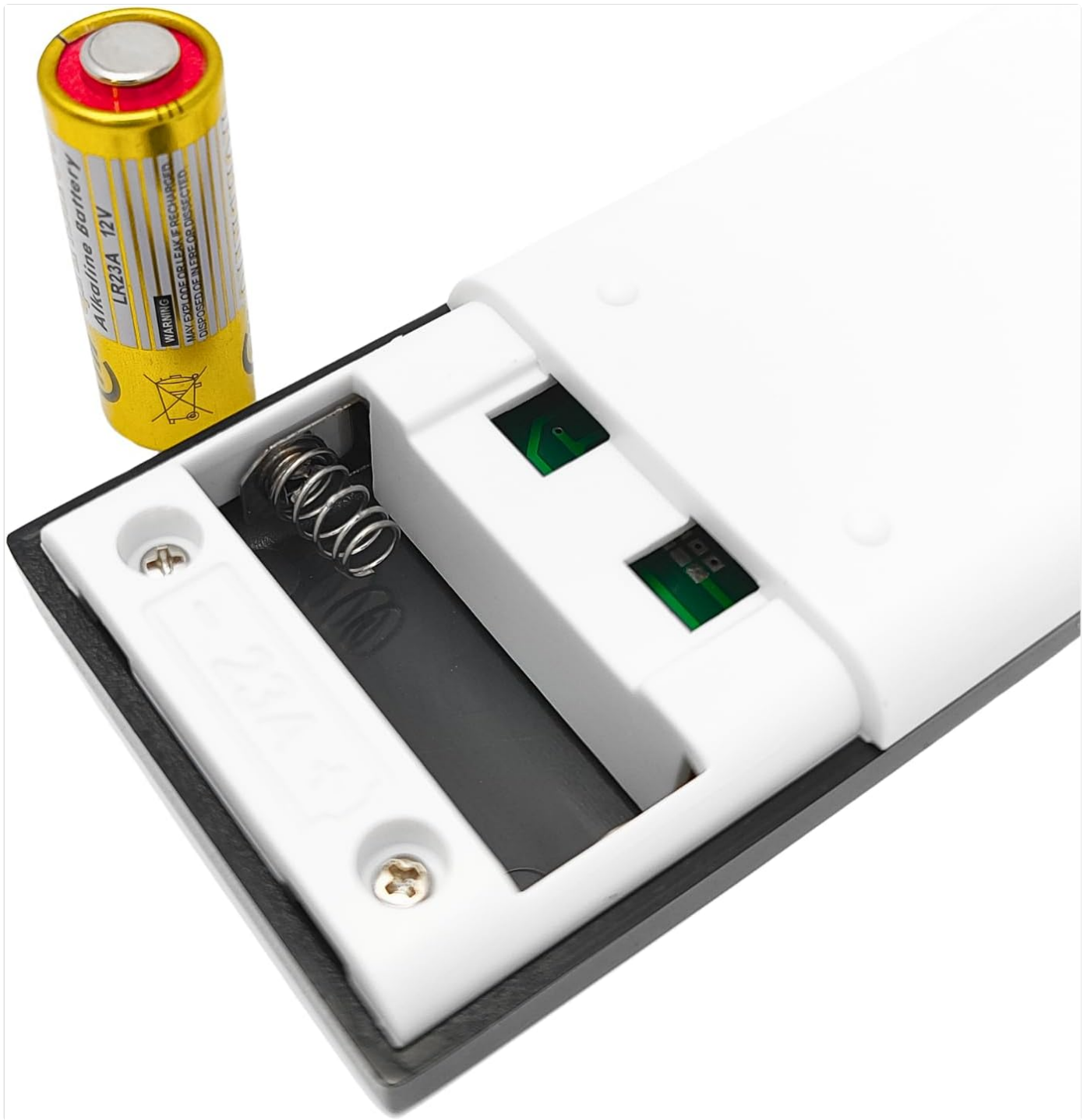
Figure 2.3: The remote control with its battery compartment open, showing the required 12V LR23A battery.
