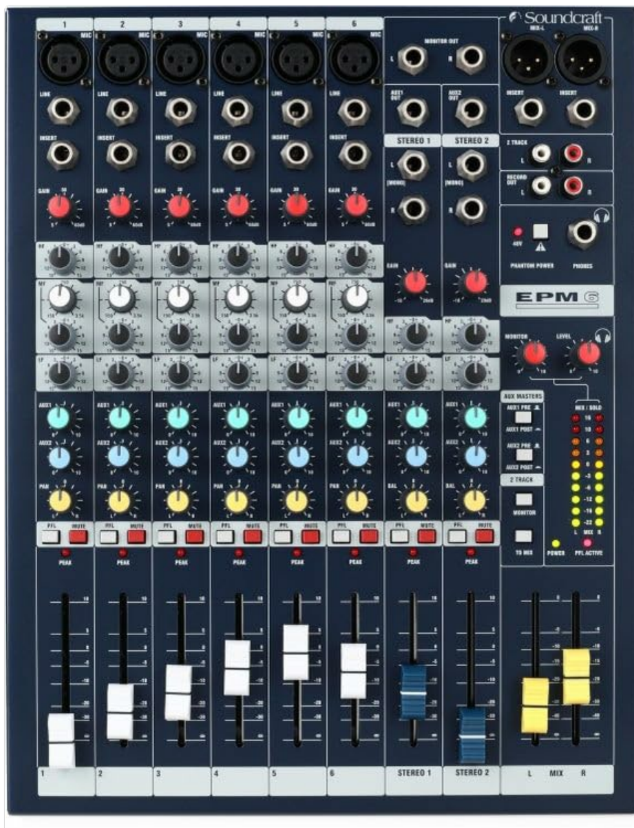
Figure 1: Front view of the Soundcraft EPM6 mixer, showing input/output sections and channel controls.
