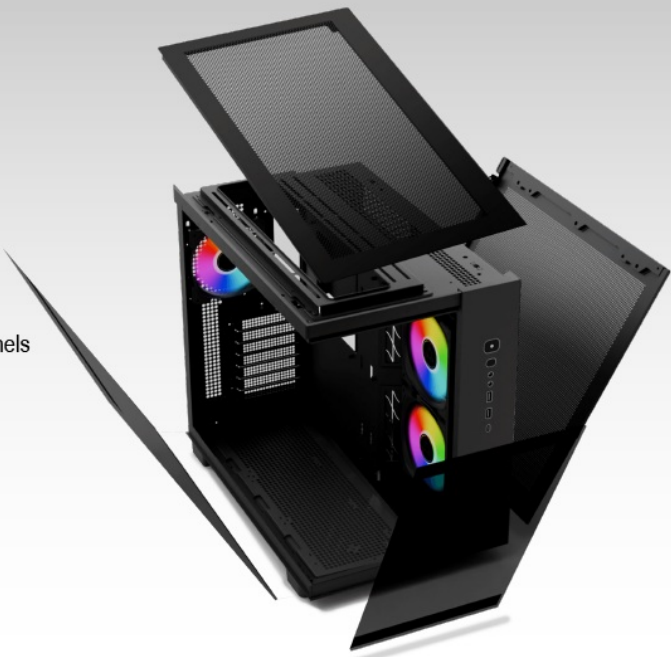
Image 5.1: The case's design highlights efficient ventilation through its mesh panels.
