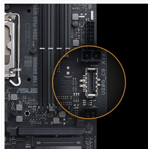
Figure 7: Detail of a USB header for connecting front panel USB ports.
