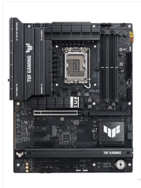
Figure 3: Overview of the motherboard layout, showing the LGA 1851 CPU socket.
