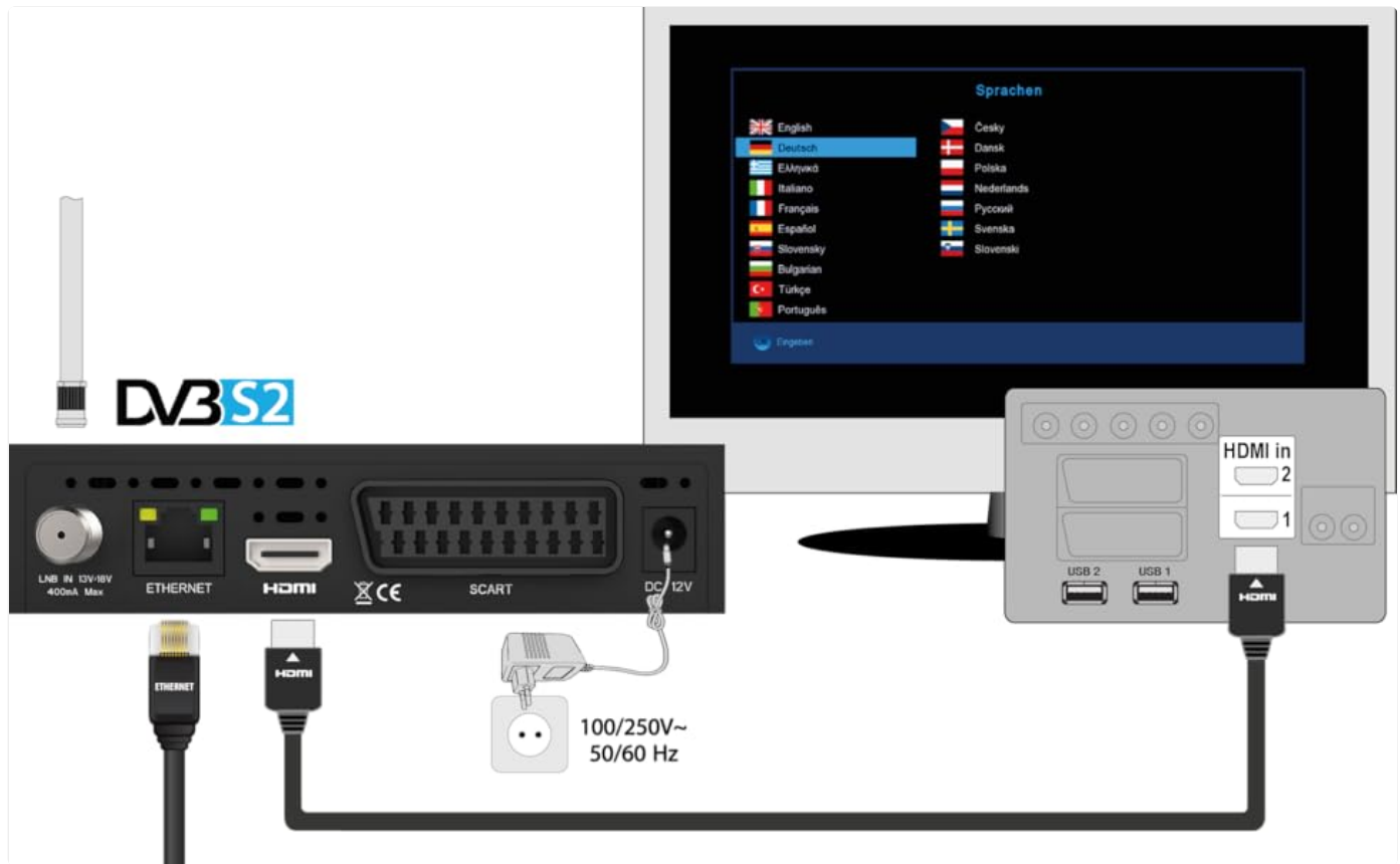
Image: An illustrative diagram demonstrating how to connect the satellite receiver to a television using an HDMI cable and the power adapter, along with an optional WiFi dongle.
