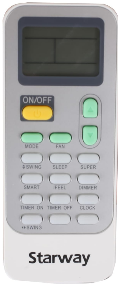
Figure 3: Starway Air Conditioner Remote Control. This image shows the remote control with clearly labeled buttons for various functions such as ON/OFF, Mode, Fan, Swing, Sleep, Super, Smart, IFeel, Dimmer, Timer On, Timer Off, and Clock.
