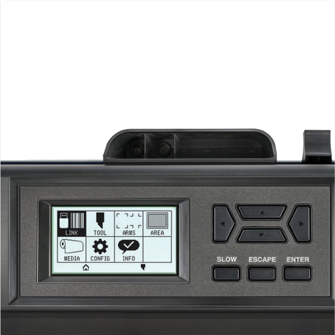
Figure 5.1: The plotter's control panel, showing the touch screen display and navigation buttons.
