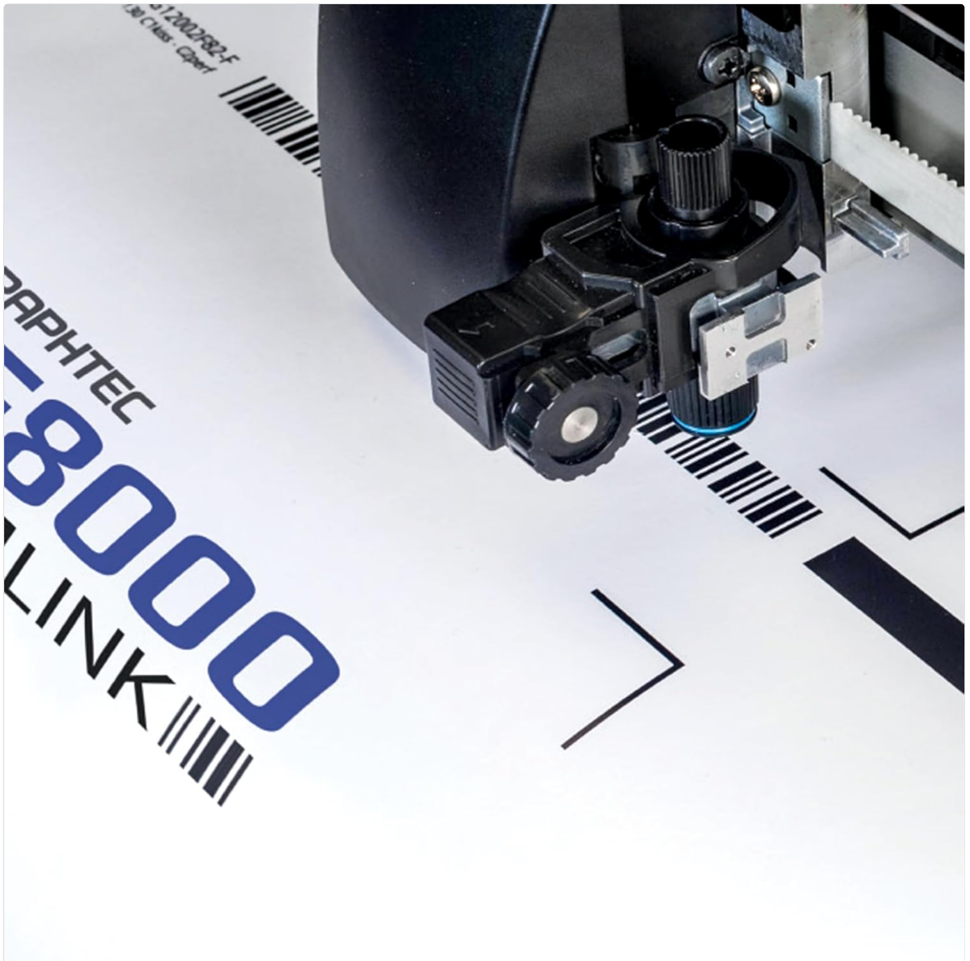
Figure 5.2: The cutting head precisely reading registration marks on printed media for accurate contour cutting.
