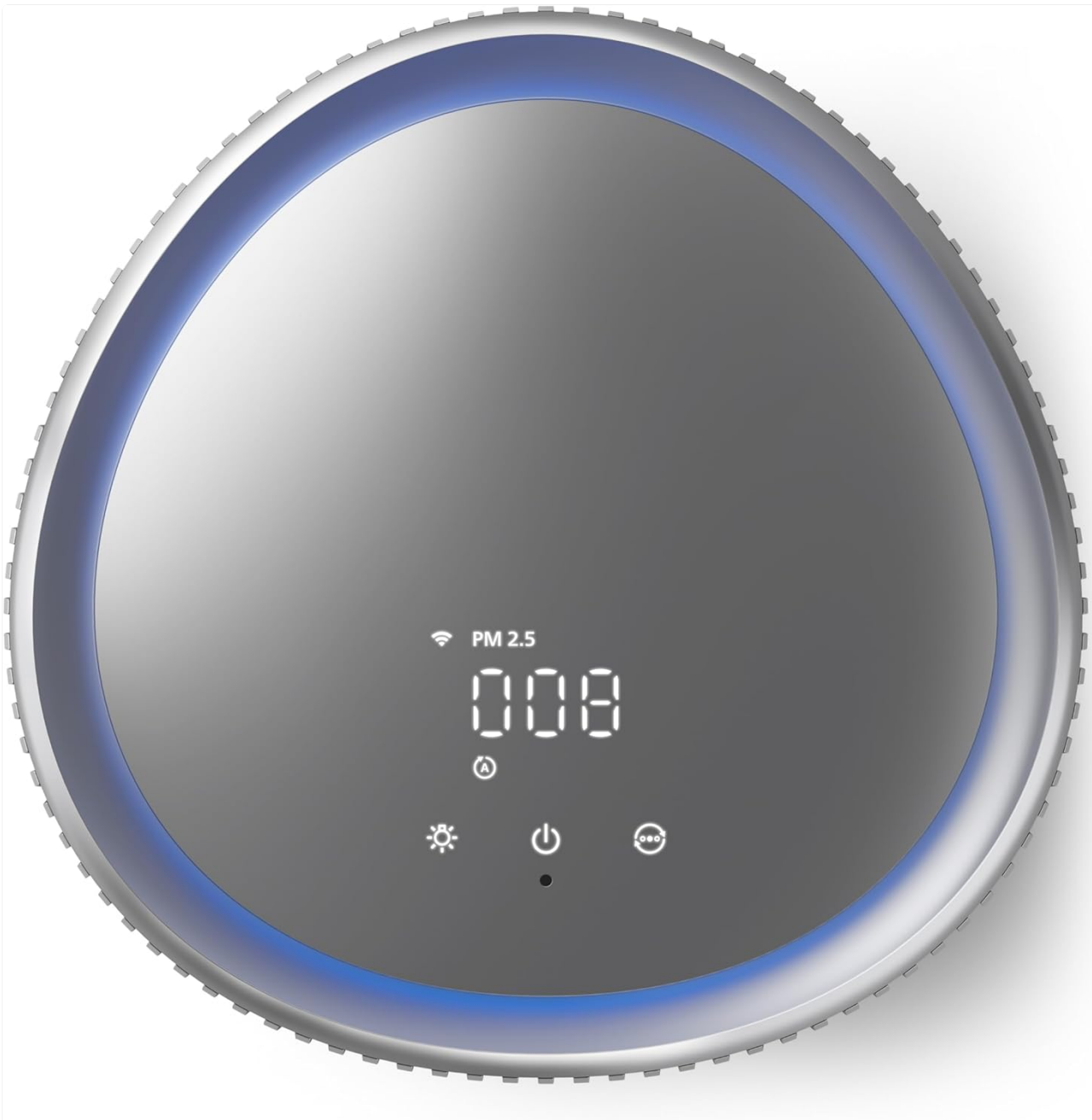
Figure 4: Top control panel with digital display and touch buttons.
