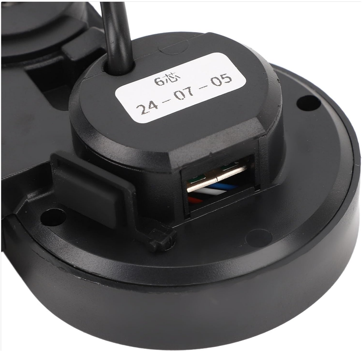
Figure 4: Detailed view of the 6-pin connector
