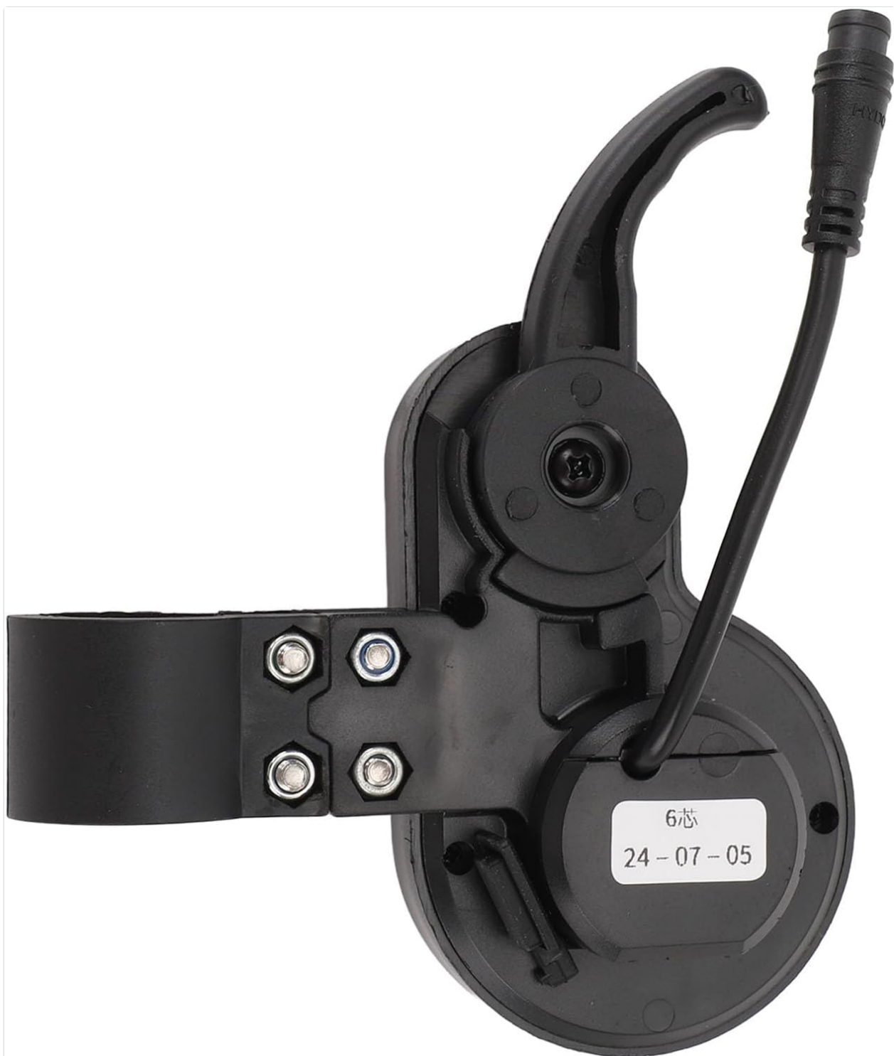
Figure 3: Rear view of the TF 100 unit with the 6-pin connector
