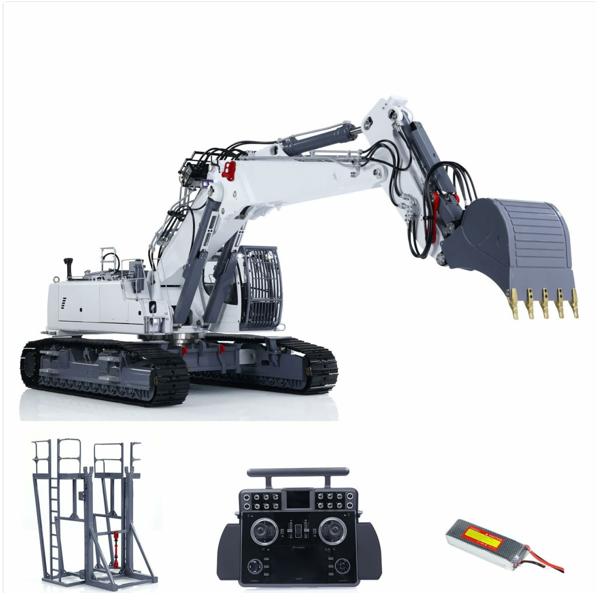
Figure 1: Front-side view of the LESU LR960 1/14 RC Hydraulic Excavator with its arm extended and bucket attached.
