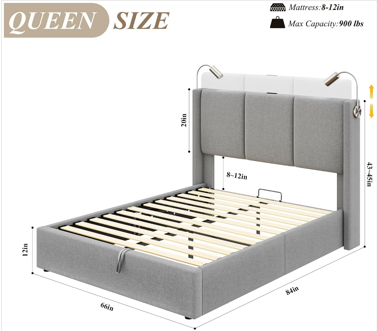
Image: Dimensional drawing of the Queen size bed frame, indicating length, width, and height measurements.
