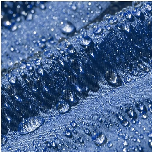
Image 7.1: The tent's waterproof fabric with PU2000mm coating, designed to repel rainwater.
