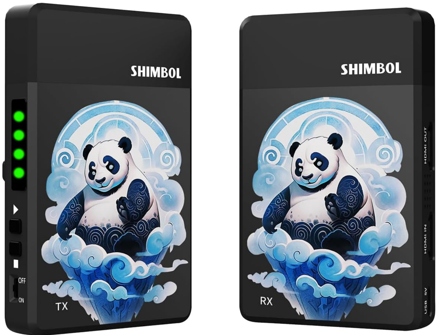
Image 4.1: Front view of the Shimbol TP Max Transmitter (TX) and Receiver (RX) units, showing their compact form factor and indicator lights.
