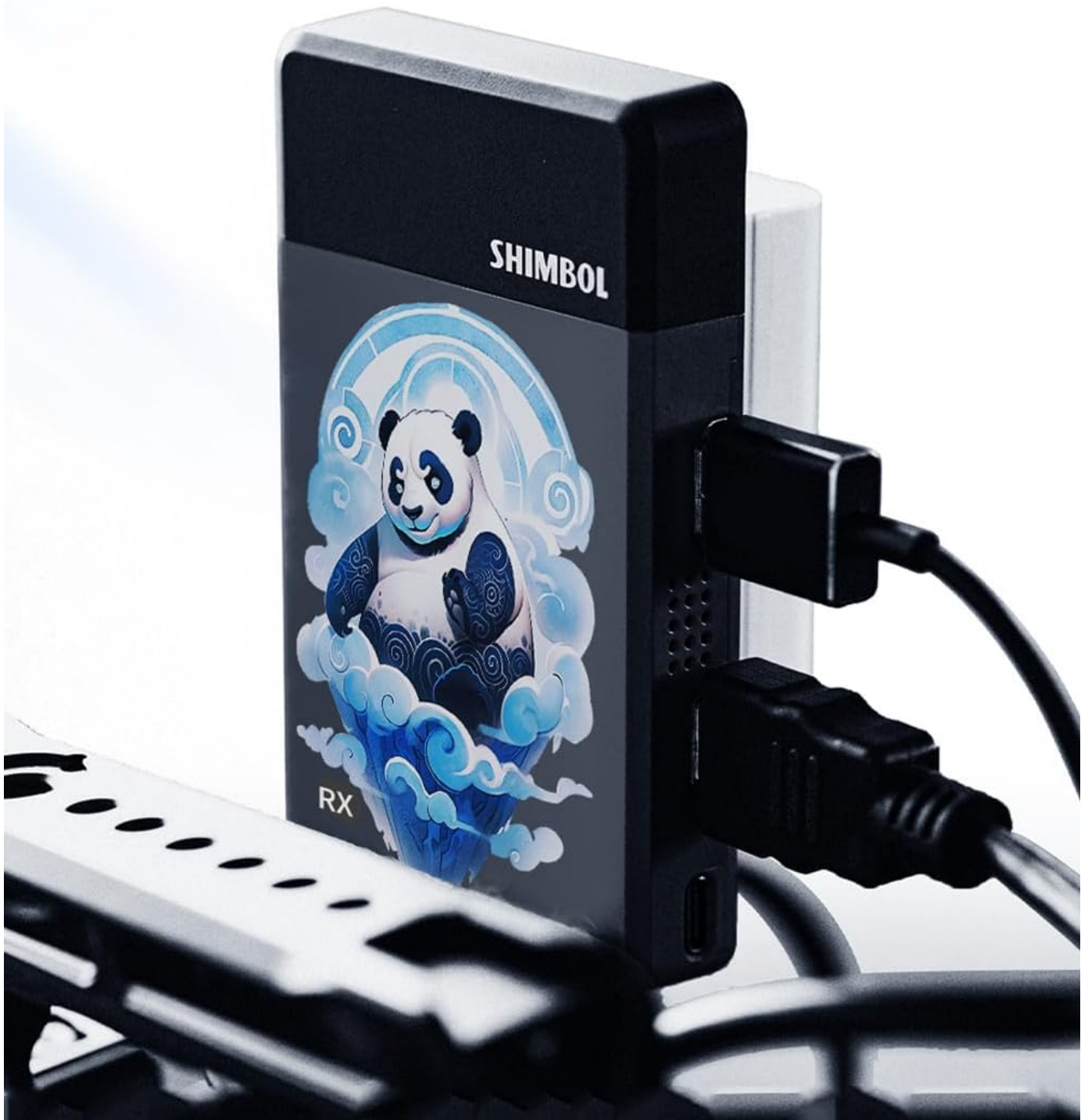
Image 4.2: Side view of the Shimbol TP Max Receiver (RX) unit, illustrating the HDMI IN/OUT ports and USB-C power input.
