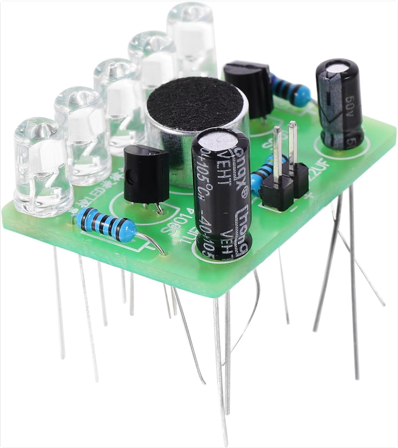
Image: A detailed view of the Sound Activated LED Lamp Module, showcasing its compact design and integrated components including the microphone and LEDs.
