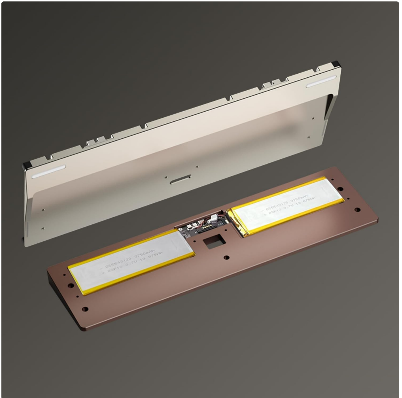
The internal layout of the keyboard, revealing the dual battery setup for extended power.
