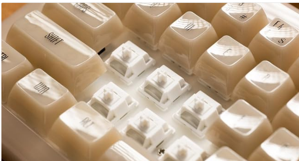
Figure 6: Close-up view of the hot-swappable sockets on the Akko YU01 keyboard, with keycaps removed.
