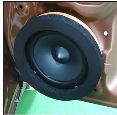
Image 2.1: Detailed product dimensions showing outer diameter of 7.7 inches and inner diameter of 5.7 inches.
