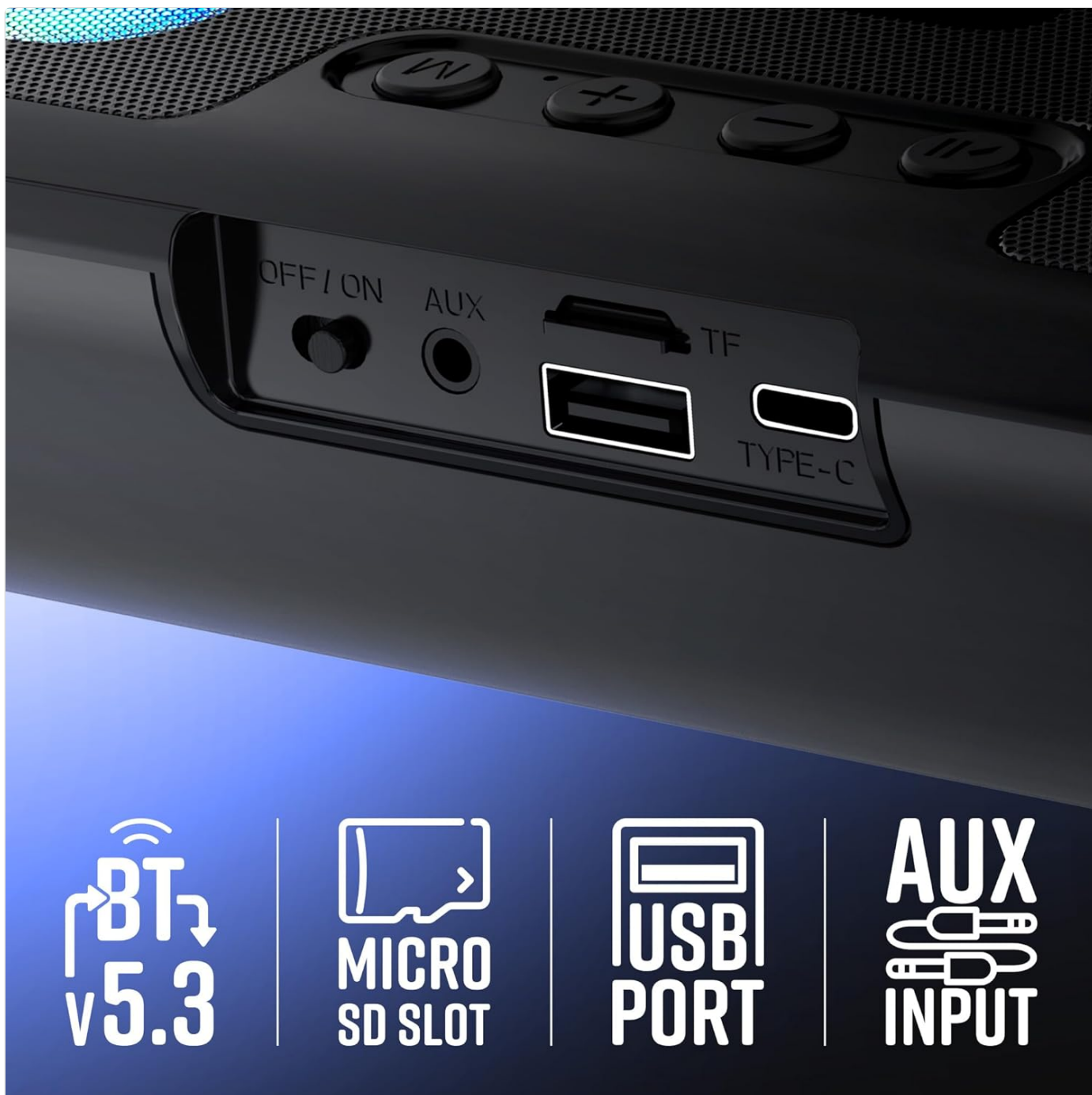
Image: Detailed view of the speaker's connectivity panel, showing the power switch, AUX, USB, microSD (TF), and Type-C charging ports, alongside icons illustrating its various connectivity options.
