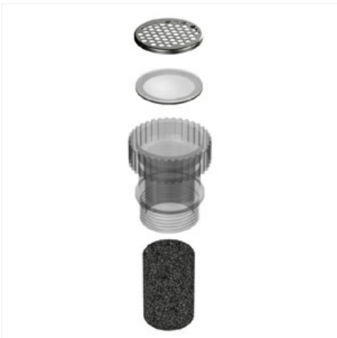
Image: An exploded view showing the individual components of the nozzle assembly, including filters and mesh.
