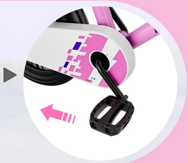
Coaster Brake Pedal backwards to stop
