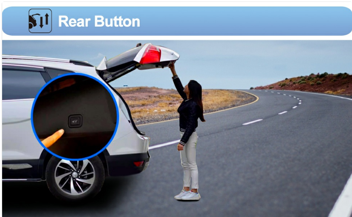
Image 5.3: A hand pressing the button located on the tailgate to close it.
