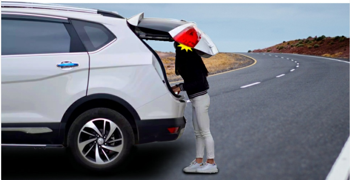
Image 5.6: An illustration demonstrating the anti-pinch feature of the power liftgate, where the tailgate reverses upon detecting an obstruction.
