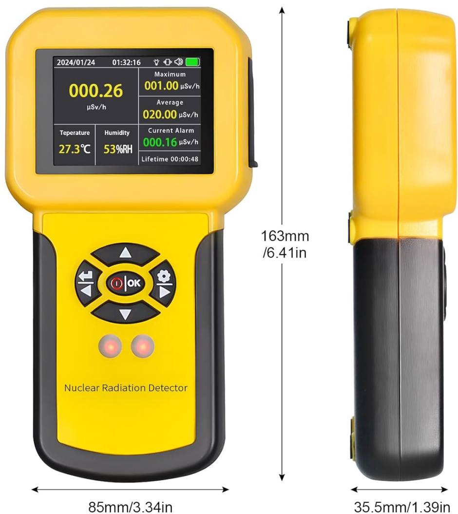
Figure 8.1: Physical dimensions of the AP-886A detector.
