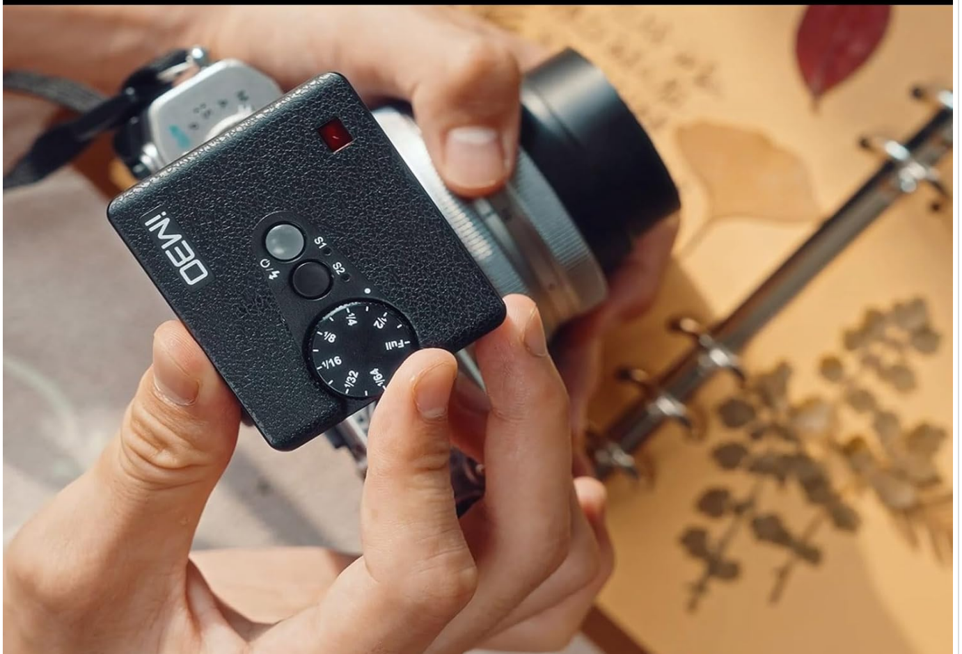
Figure 5: Adjusting flash power. A hand is shown turning the power dial on the Godox iM30 flash unit.
