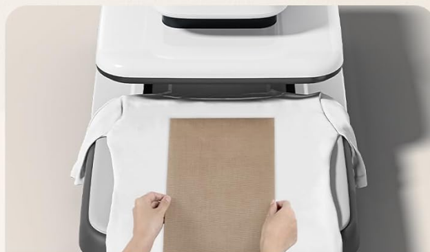
Step3: Place the substrate, material, and Teflon sheet in order
