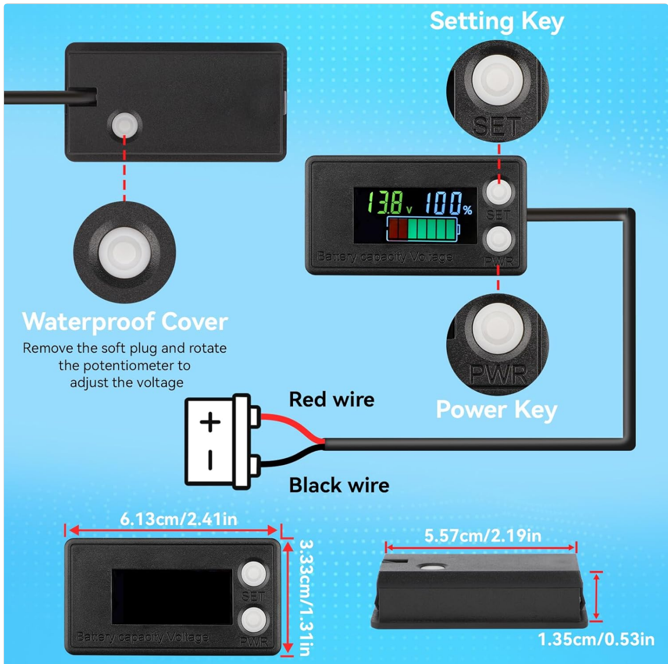
Figure 3: Wiring diagram and physical dimensions of the DROK Battery Monitor.
