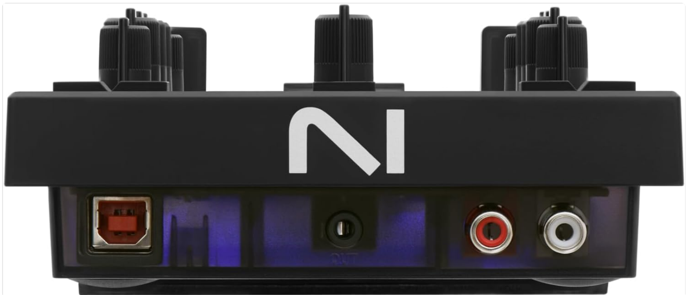
The rear panel of the Z1 Mk2, featuring the USB port for computer connection and audio output jacks.
