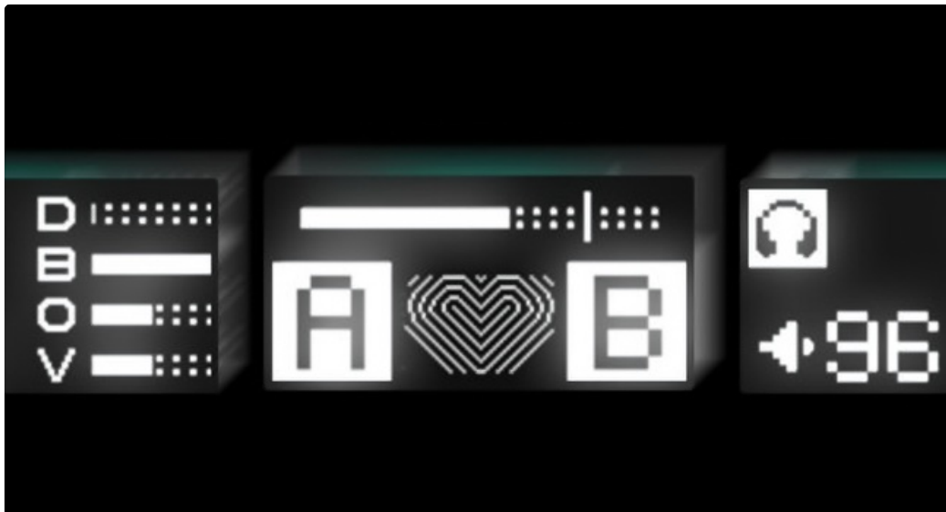
The three OLED displays providing real-time visual feedback on mixing parameters.
