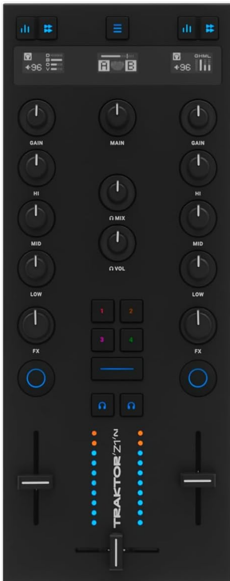
A comprehensive view of the Z1 Mk2's control surface, including knobs, faders, and buttons.
