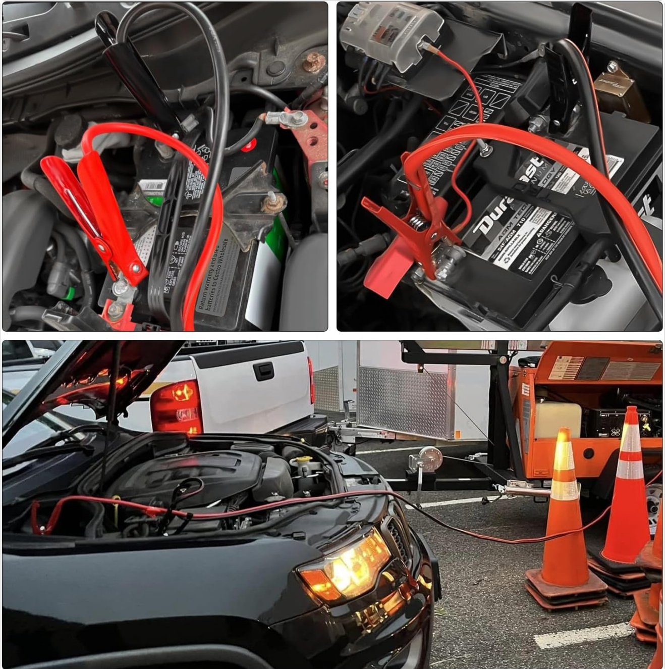
Image 4.2: Examples of jumper cables connected to vehicle batteries and engine components during a jump-start.
