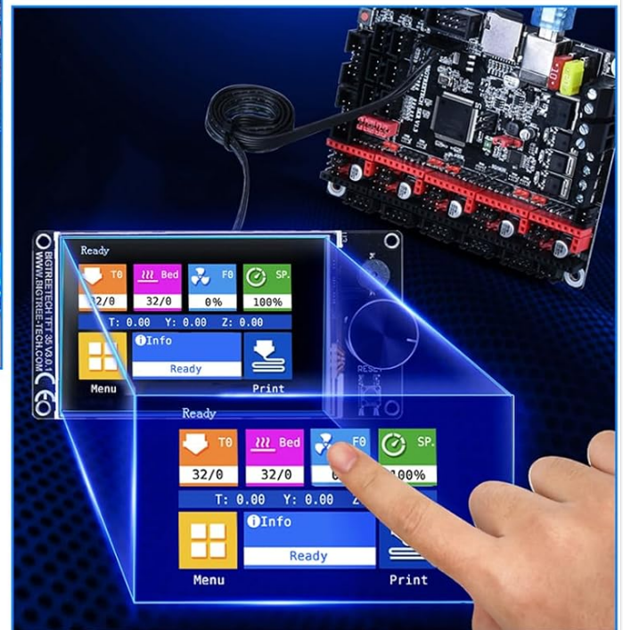
Figure 3.2: TFT35 V3.0.1 Display Modes. This image illustrates the two operational modes of the TFT35 V3.0.1 display: the traditional 12864 LCD mode and the modern Serial Touch Screen mode, along with their respective connection methods.
