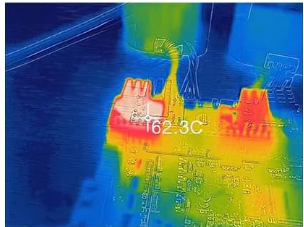
Figure 5.1: TMC2209 Thermal Management. This image highlights the large-area fan thermal pad on the TMC2209 driver, designed to reduce heat dissipation temperature, along with thermal imaging examples.
