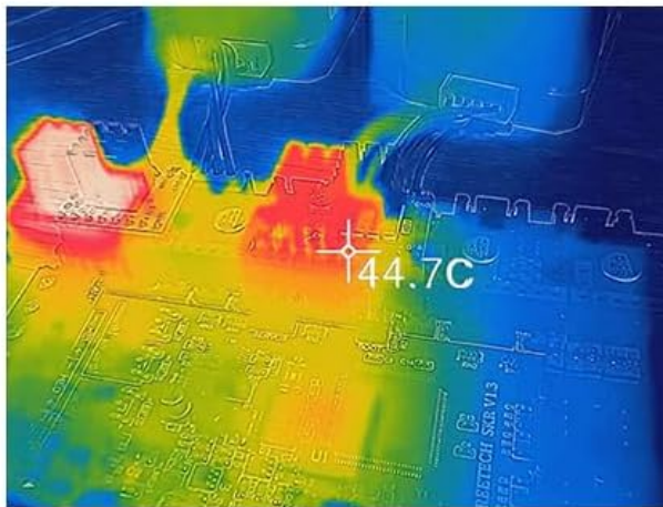
Figure 5.1: TMC2209 Thermal Management. This image highlights the large-area fan thermal pad on the TMC2209 driver, designed to reduce heat dissipation temperature, along with thermal imaging examples.
