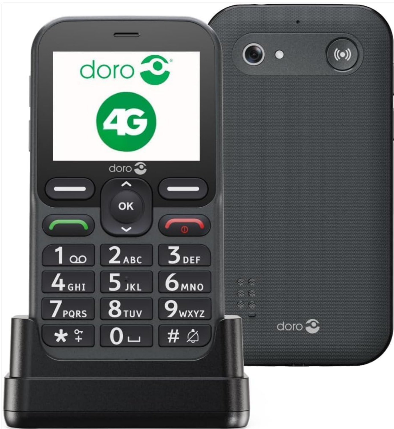
Figure 1: Doro Leva L10 mobile phone with its charging dock, showing both the front keypad and screen, and the textured back panel with camera and assistance button.
