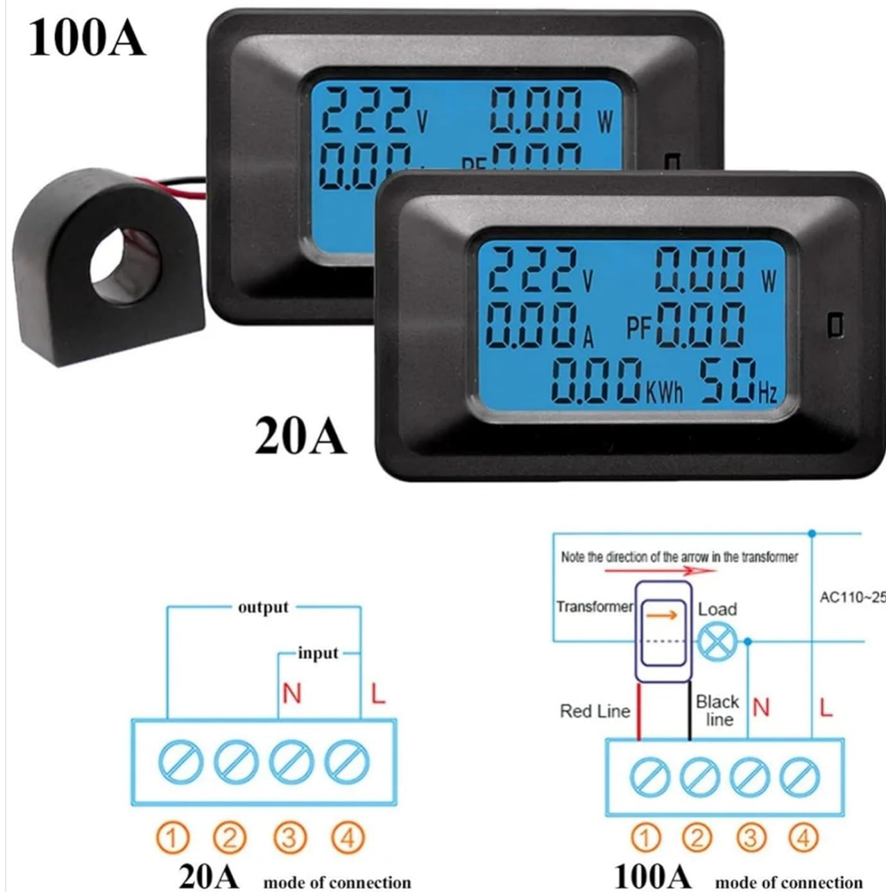
Figure 3: Connection diagrams for both 20A (left) and 100A (right) models. Note the direction of the arrow on the transformer for the 100A model.
