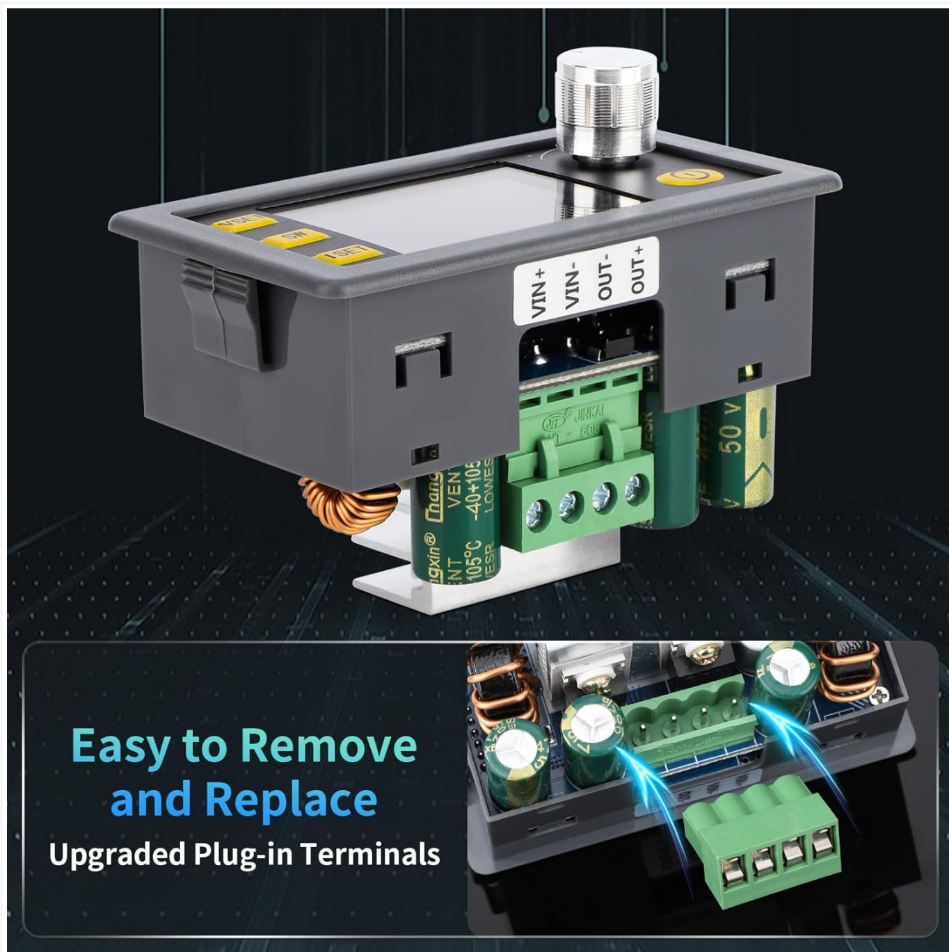
Figure 5: The upgraded plug-in terminals facilitate easy and secure wiring.
