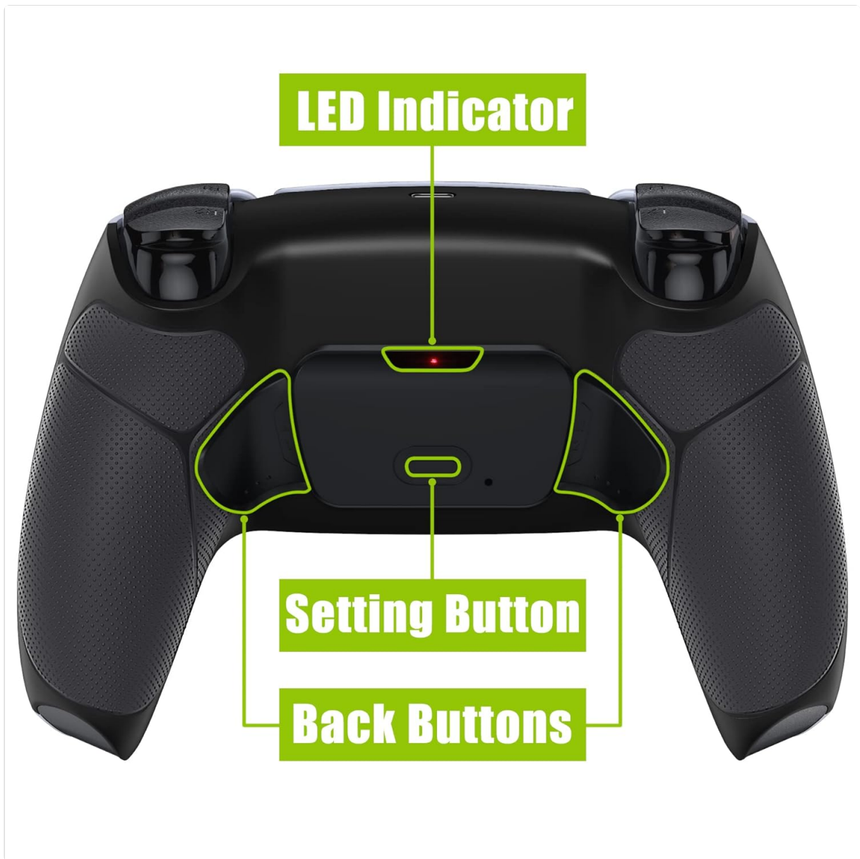
Image: PS5 controller with the RISE V3 Remap Kit installed, highlighting the back buttons and LED indicator.
