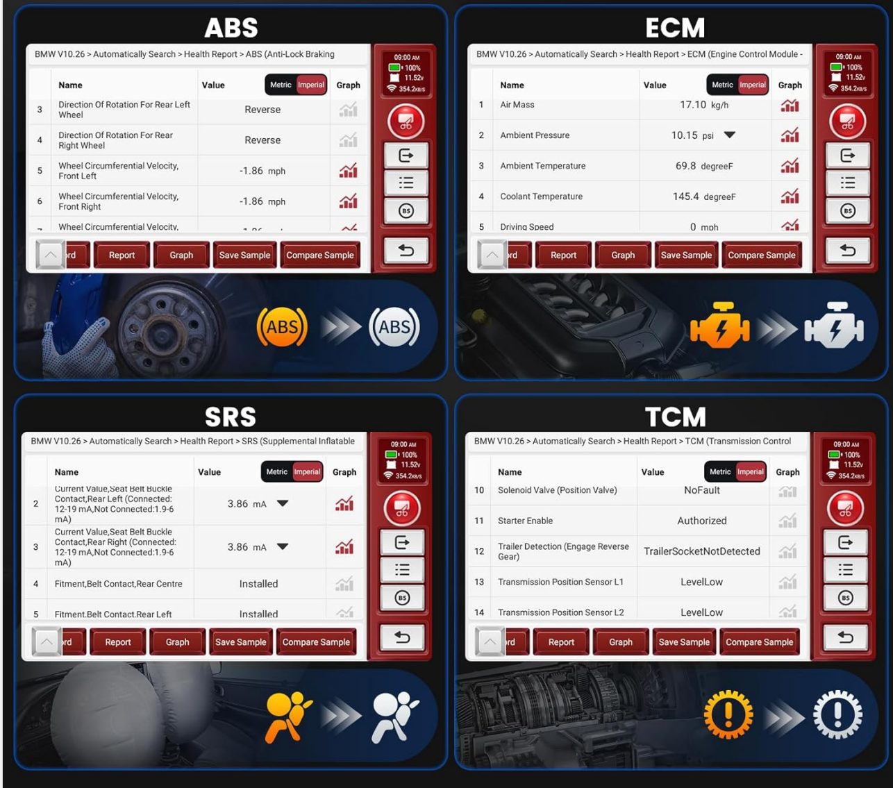
Figure 3.7: Example of real-time data streams for ABS, ECM, SRS, and TCM.
