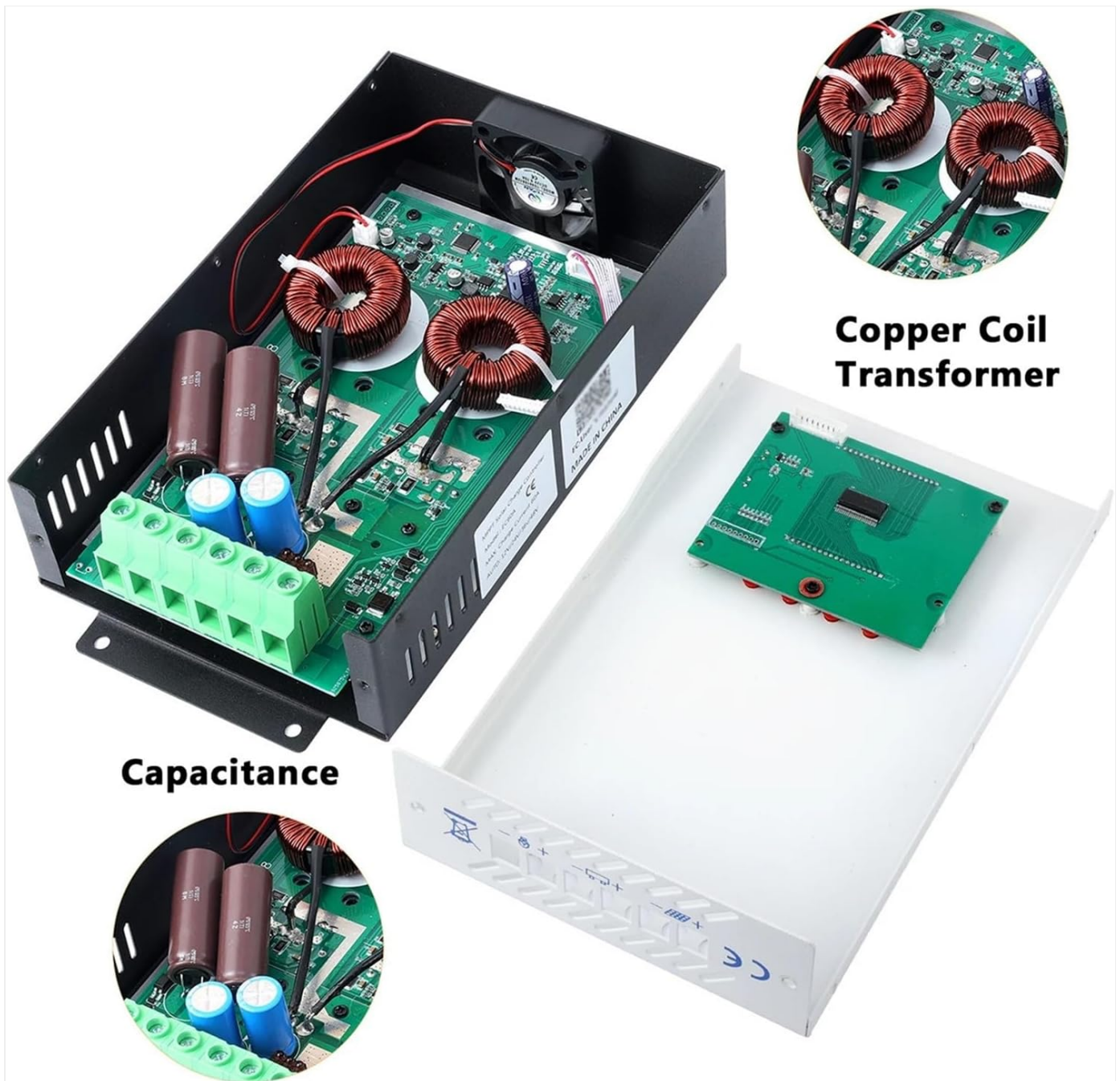
Figure 4: Internal view of the controller, highlighting key components such as capacitance and copper coil transformers, indicative of robust construction.
