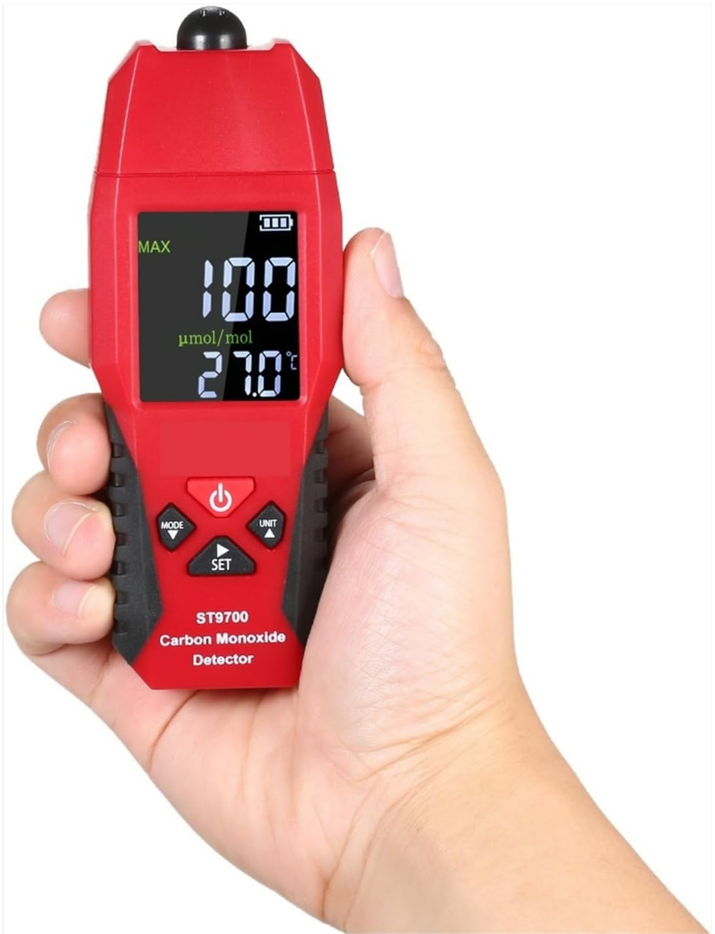
Figure 4: The ST9700 meter displaying a CO reading and temperature.
