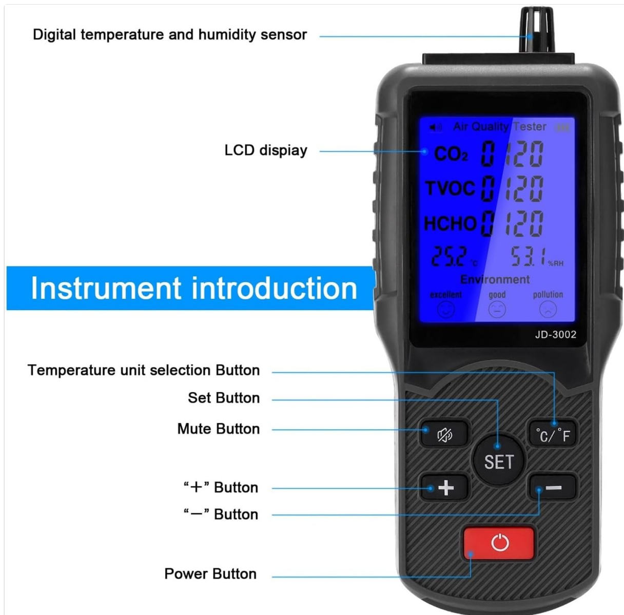
Figure 2.2: Diagram illustrating the main components and buttons of the JD-3002 Air Quality Monitor.
