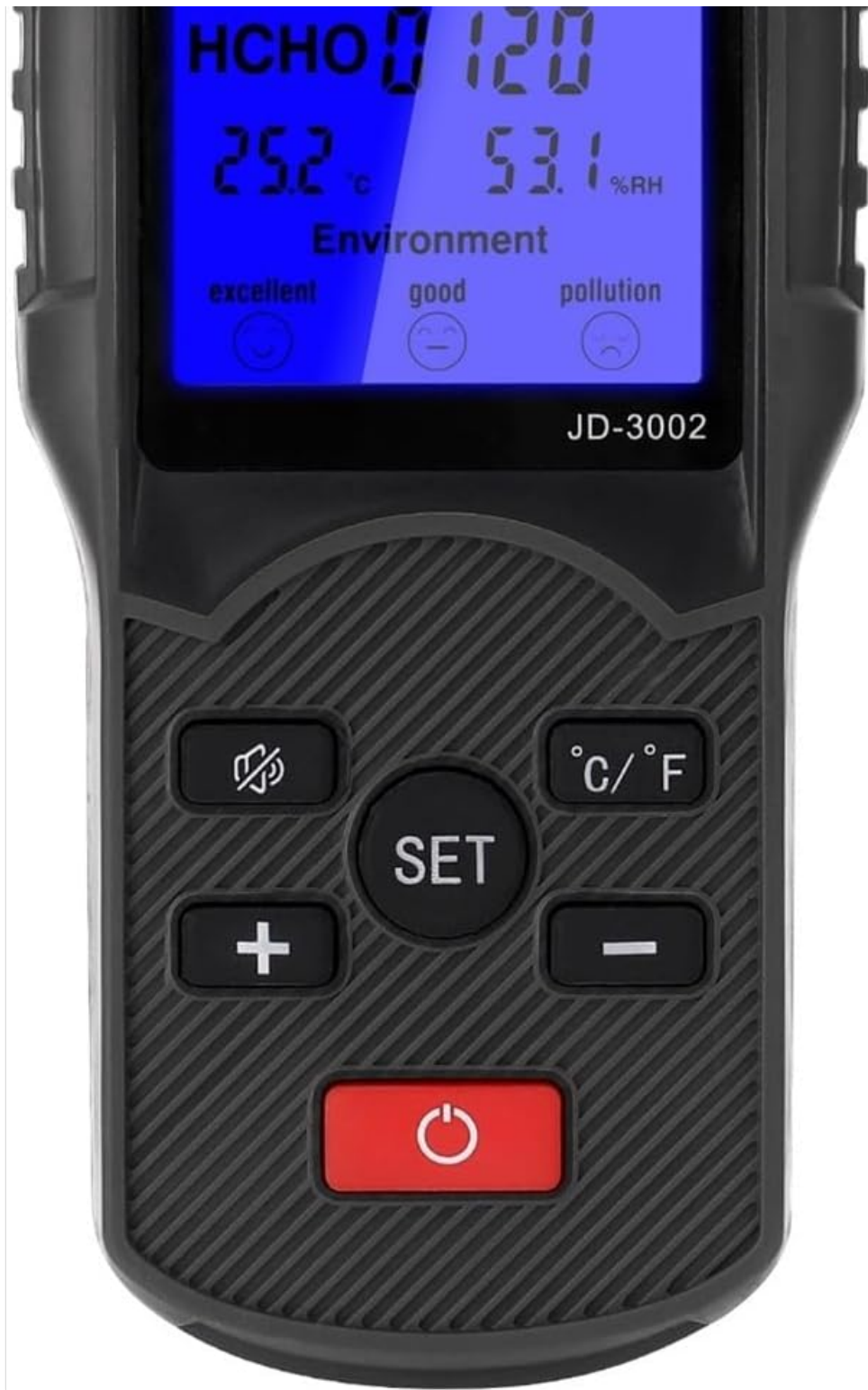
Figure 2.1: Front view of the KYKYK JD-3002 Air Quality Monitor, showing the display and control buttons.
