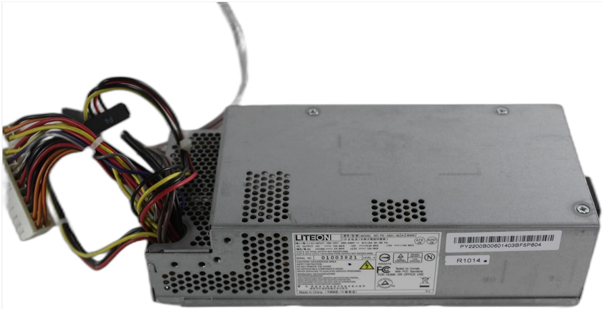
Image 1: Top view of the PSU, showing the model label and safety warnings. The label indicates Model No. PS-5221-06A1 ROHS, AC Input 100-127V / 220-240V, and various DC outputs. It also displays safety certifications and warnings against opening the unit.
