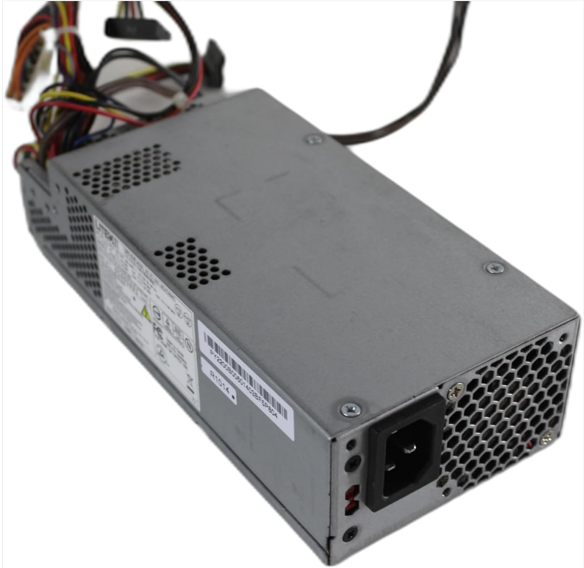
Image 3: Rear view of the PSU, highlighting the AC power input socket and the ventilation grille. This is where the main power cable connects to the unit.
