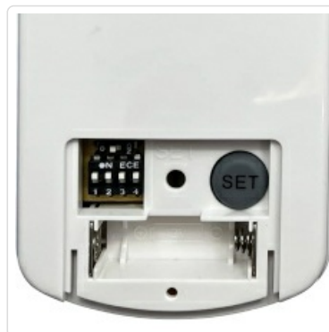
Image: Close-up of the remote control's battery compartment, showing the slot for the 23A/12V battery and the dip switches.
