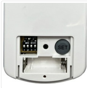
Image: A detailed view of the dip switches located within the remote control's battery compartment, ready for setting a code.
