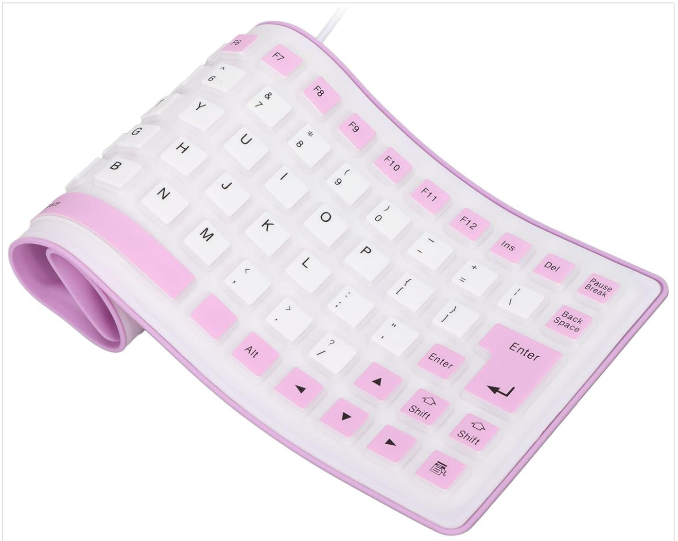
Figure 5: A clear view of the 85-key layout of the silicone keyboard.
